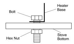
Figure 14 - Fastening Heater Base to Stove Drop Bottom
